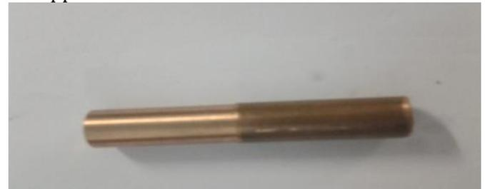
Fig: 4.2 copper electrode
